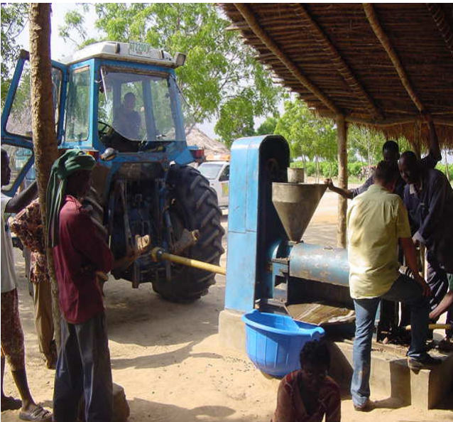
Photo 3: Tractor-Mill connection for Oil extraction
